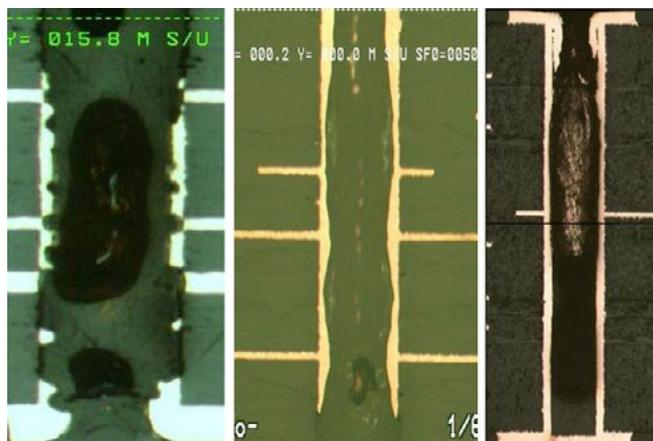
Figure 4: Typical defects detected using 4-Wire Kelvin.
