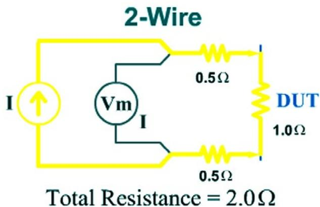
Figure 2: Two leads with 0.5 ohms resistance.
